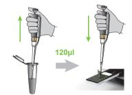
6. After applying the sample, immediately press the TEST START' button.
